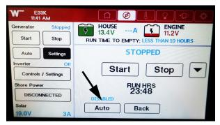
The Auto Operation Condition is displayed as Enabled, Disabled, or Locked out. -Typical View
