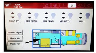
Selecting this zone controls the hall, middle math, bed ceiling, bed reading, and rear bath light. -Typical View
