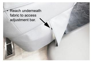
The Driver and the Passenger seats both have an adjustment bar under the fabric in the front. Pull up to slide the seat forward or rearward. -Typical View
