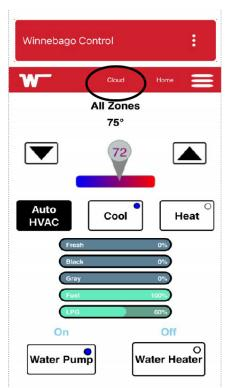
11. When the "Cloud" indicator is displayed at the top you are using the app in the "Farfield" operating mode. -Typical View
