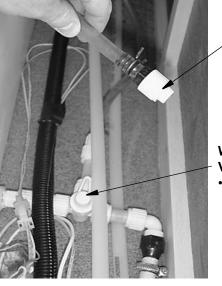
Antifreeze Siphon Tube • Insert into container of RV water system antifreeze
