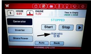
After selecting the generator button the hourmeter will display. -Typical View
