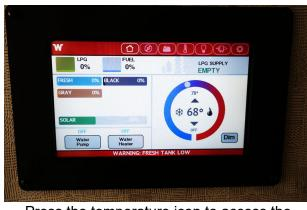
Press the temperature icon to access the climate screen. -Typical View
