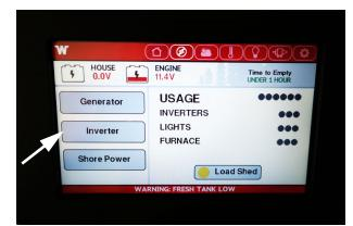
From the main menu select the battery section and the screen with the inverter button will show in the menu. -Typical View
