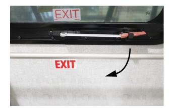
Escape Window Lift up on the bar slightly to clear the retention latch, then pull the bar straight towards the inside. -Typical View
