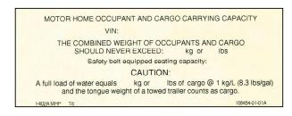
If any weight exceeding 45.4 kg (100 lbs.) is added to your motorhome between final vehicle certification and first retail sale, the occupant and cargo carrying capacity must be corrected and a label similar to the one shown in the following photo will be affixed inside your motorhome.
