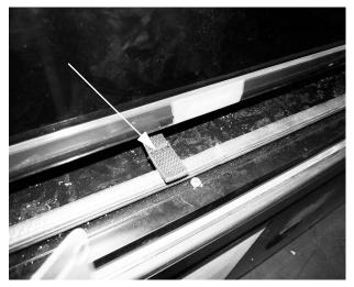
To adjust the TV, pull the black strap (located on back side of TV) straight down to release the TV from the mounting bracket. -Typical View
