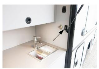
Tailgate Sink Drain Pump Switch (Located near exterior (tailgate) sink) -Typical View
