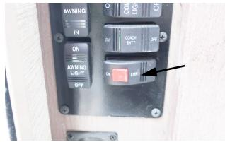
Entry Step Switch Located near entrance door (The switch configuration may vary) -Typical View
