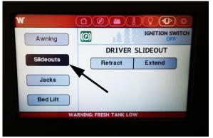
From the slideout/awning screen select the slideout button to access the slideout controls. -Typical View
