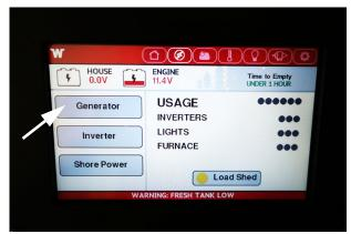
From the main menu select the electrical section and the screen with the generator button will show in the menu. -Typical View
