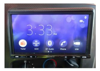
Main Menu Screen with radio tuner, SXM satellite tuner, Bluetooth audio, phone and USB options. Press the Home button at any time to return to the main menu. -Typical View
