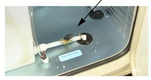
Waterline and Water Tank Drain Valves -Typical installation shown (See the "Water System Drain Valve Locations" chart at the end of this section for locations on your model)
