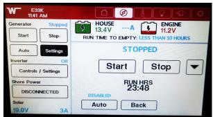
Generator Settings Screen Use this screen to customize various triggers to automatically start and stop the generator. Select the down arrow for further customizations and options. The total run hours are also displayed on this screen. -Typical View
