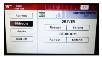
Slide-out Controls After reading the warning message, click on the accept button to access the slide-out controls. Refer to the slide-out section in the slide-outs and leveling chapter in this manual for operating instructions and safety precautions. -Typical View
