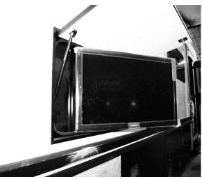
Pull the TV out and pivot to desired position. To return to storage, rotate TV back to center position and press straight back. You will hear a "click" when the TV is secured into locked position. -Typical View
