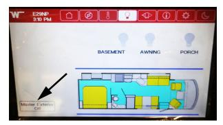
Pressing the Exterior Lights button will reveal the buttons that control the awning, porch, and basement lights. (The basement light command must be turned on for the basement lighting to be powered). -Typical View
