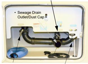
Gray Waste Tank Drain Valve  Black Waste Tank Drain Valve
