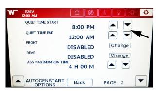
Page 2 of the AGS shows the quiet time start and end settings (local time is used to prohibit starting the genset during quiet time settings. -Typical View
