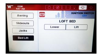
Bed-lift Controls After reading the warning message, click on the accept button to access the bed-lift controls. Refer to the power loft bed section in the furniture and softgoods chapter in this manual for operating instructions and safety precautions. -Typical View
