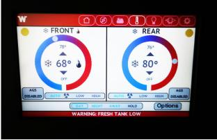
Use the up and down arrows to adjust the front and the rear of the motorhome to the desired temperature. -Typical View
