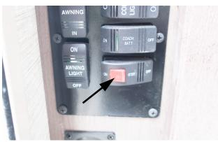
Red Activation Lever • The red Activation Lever located on the entry step switch must be depressed in order to put the step switch in the ON position. (The switch configuration may vary) -Typical View
