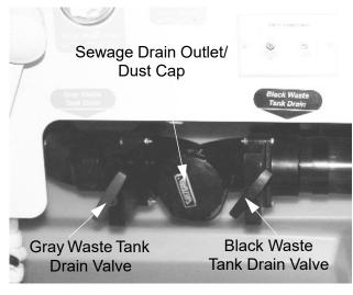
Holding Tank Drain Valves (Located in water service center) -Typical View Black and Gray Waste Tank Drain Valve positions may be reversed, depending on floorplan and tank location.  Tailgate Package Waste Drain Valve (If Equipped)
