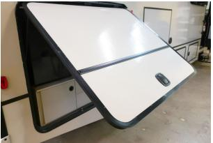
Pull the door latch to open the compartment door. The door will stop at this position.
