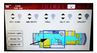
Selecting this zone controls the galley, galley overhead, hall, middle bath and bed ceiling lights. -Typical View
