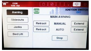
Awning Controls After reading the warning message, click on the accept button to access the awning controls. Refer to the awning section in the miscellaneous chapter in this manual for operating instructions and safety precautions. -Typical View
