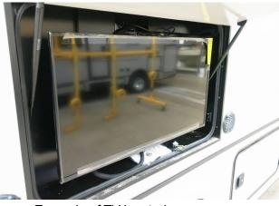
Example of TV located on passenger side lift up panel. -Typical View
