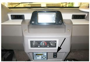
Radio Power Switch (Located on lower dash area)
