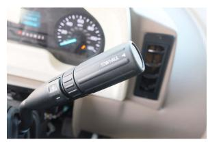
Press the button at the end of the shift lever to engage Tow/Haul Mode when pulling a trailer or tow vehicle.
