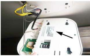
Factory SSID and password shown on the back of the router. (Located on the coach ceiling). -Typical View
