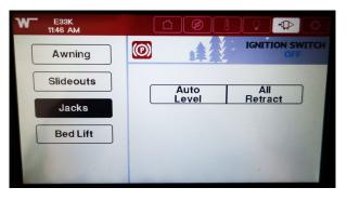
Leveling Controls After reading the warning message, click on the accept button to access the leveling controls. Refer to the leveling section in the slide-outs and leveling chapter in this manual for operating instructions and safety precautions. -Typical View
